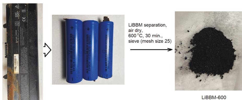
Figure 1. Preparation of the LiBBM-600 catalyst from a spent DELL 1525 laptop battery (87 Wh, 11.1 V).
