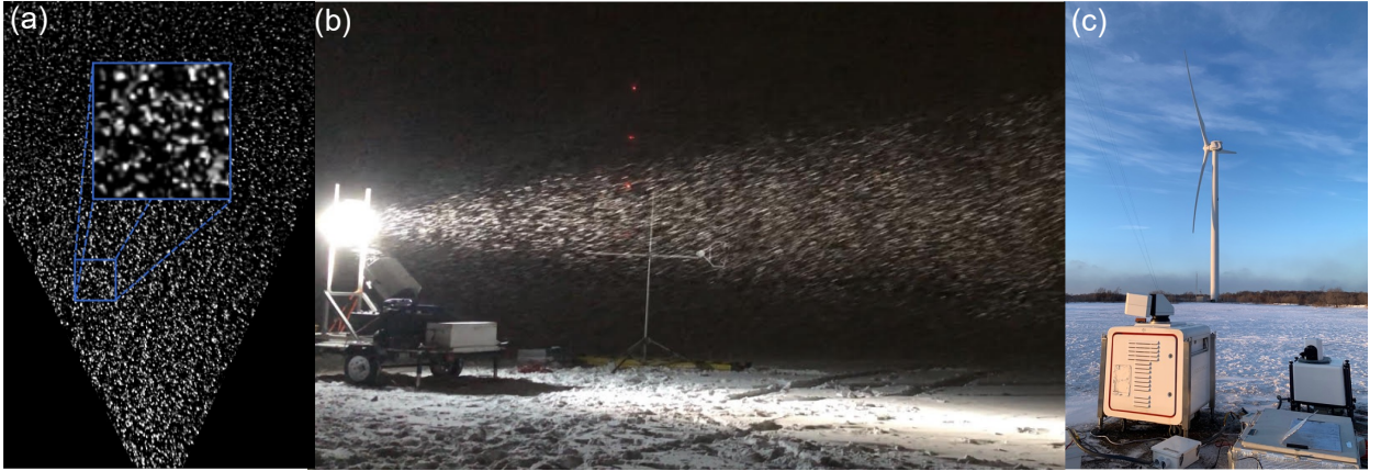
Fig. 2. Photos of the GAIA field campaign: (a) SLPIV light sheet pointing vertically; (b) SLPIV light sheet pointing horizontally; (c) deployment of the scanning Doppler LiDARs.
