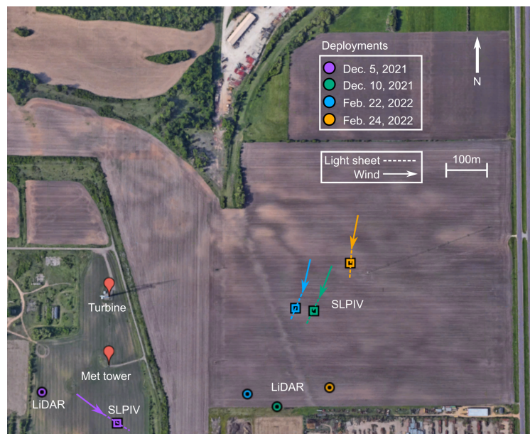
Fig. 1. GAIA field campaign at the Eolos site. Circle markers indicate LiDAR positions, square markers indicate SLPIV light sheet positions and arrows indicate mean wind directions during the deployments. Credits: Google Earth.
