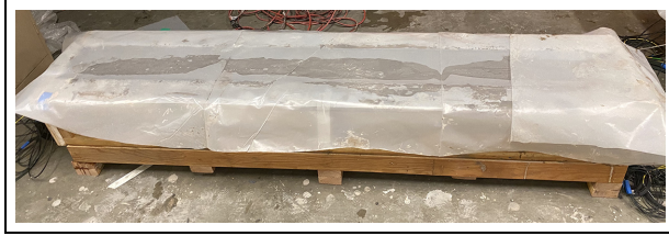
Figure 3. SCCB beam and wood mold during curing. SCCB: slag cement-cement-bentonite.
