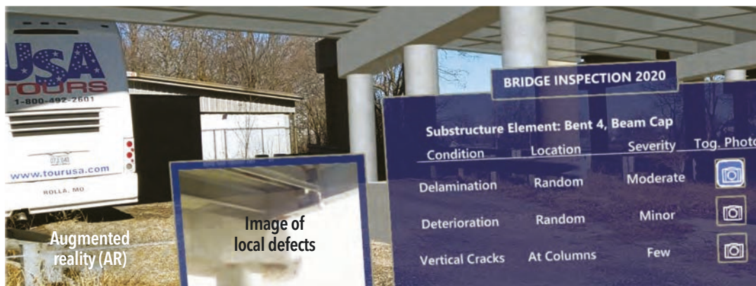
Figure 2. Hand-free bridge inspection enabled by augmented reality.
