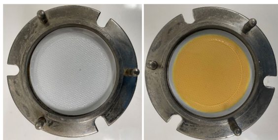
Fig. 2 CNR film deposited on an MCE support. Membrane flux is measured (left). Breakthrough data acquired by passing NaFL through the film until the C/C_0 = 1.0 . Yellow fluorescein dye of CNR is shown. (right). Regenerated films are again white
