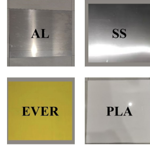
Fig. 19. Reflectors of different materials in our tests.
