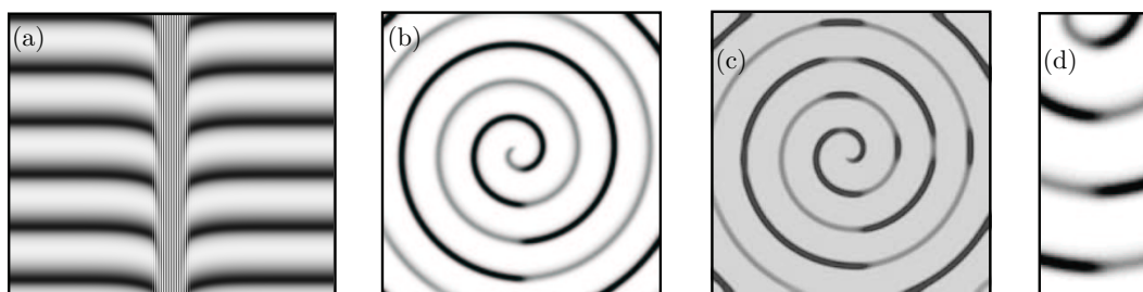
Figure 1. Panel (a) shows a space-time plot (space plotted horizontally, and time vertically) of a time-periodic solution of the one-dimensional Brusselator model: the solution exhibits a spatially periodic core in the center of the domain and spatially homogeneous oscillations in the far field away from the core region. Panels (b)–(c) contain snapshots of planar spiral waves that exhibit similar line defects (images taken from [19, 20]). Panel (d) shows an enlarged version of the spatial region around the line defect from panel (b): if we interpret the vertical direction as time, the solution resembles the space-time plot in panel (a), except that the oscillations to either side of the defect are out of phase by half the period.
