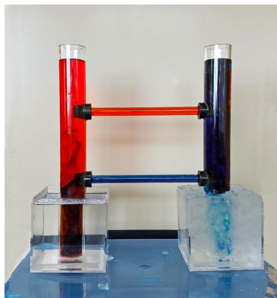
Figure 3: Demonstration of density driven circulation created by the interaction of water warmed on one side (red) and water cooled on the other side (blue).
