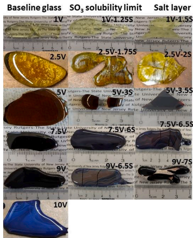
Fig. 1. Images of V_2O_5 -containing sulfur-free glasses (xV); glasses xV-yS where sulfur solubility limit has been reached; and glasses xV-yS supersaturated with sulfur showing the formation of salt layer on their surface.
