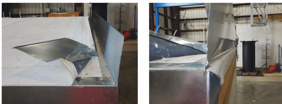
Fig. 22. Fascia and cleat lifting together at 3-sec peak wind speed of 60 m/s – configuration 4.
