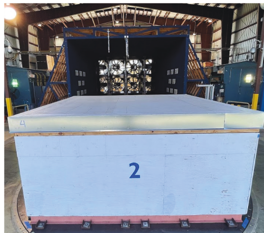
Fig. 1. Full-scale building model on WOW EF turntable.
