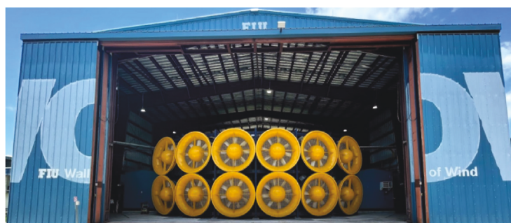
(a) 12-fan Wall of intake
