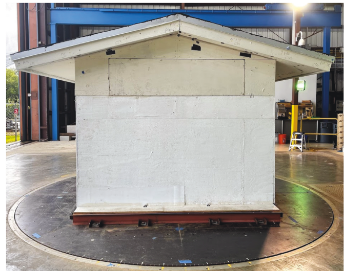
Fig. 8. Hip-gable roof at the WOW turntable.
