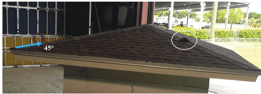
Fig. 22. Hip shingle lift at a 3-s peak wind speed of 38 m/s.
