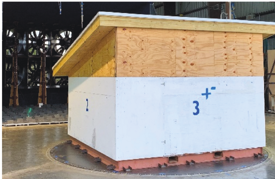
Fig. 9. Monoslope roof at WOW turntable.
