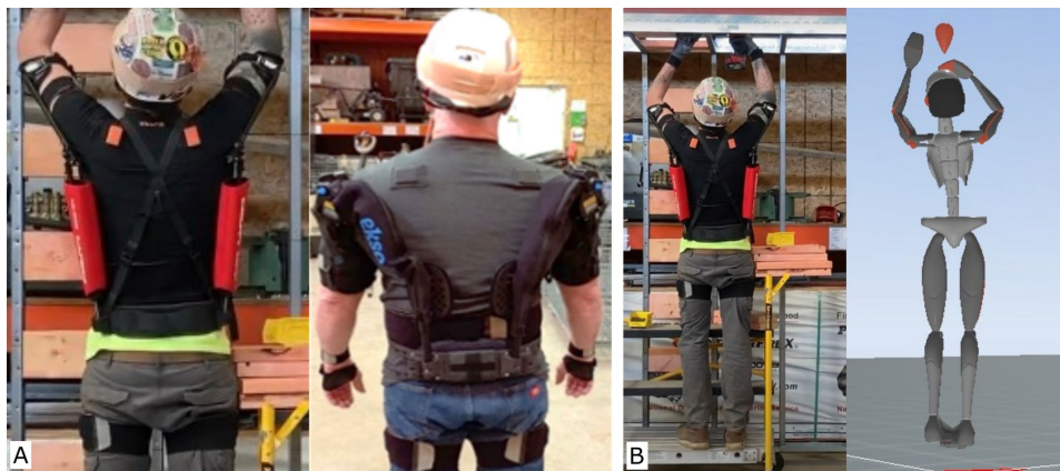
Figure 1. The two passive shoulder exoskeleton systems, and evaluation of the block removal task. A. Hilti EXO-01 (left) and Ekso Evo (right). B Still image from video data of a worker performing the block removal task (left), and a still from motion capture data from the sensor suit (right).
