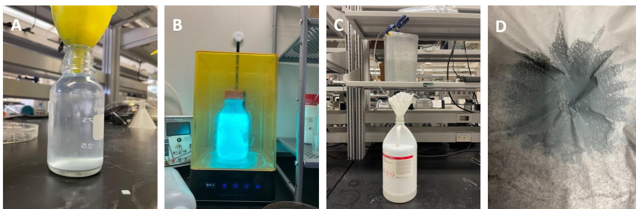
Figure 20. IPA Recycling. (A) IPA contaminated with 3D printing resin (B) exposing contaminated IPA to UV. (C) Siphoning setup used to retrieve clean IPA. (D) The residue left on the coffee filter after filtering IPA treated with alum.
