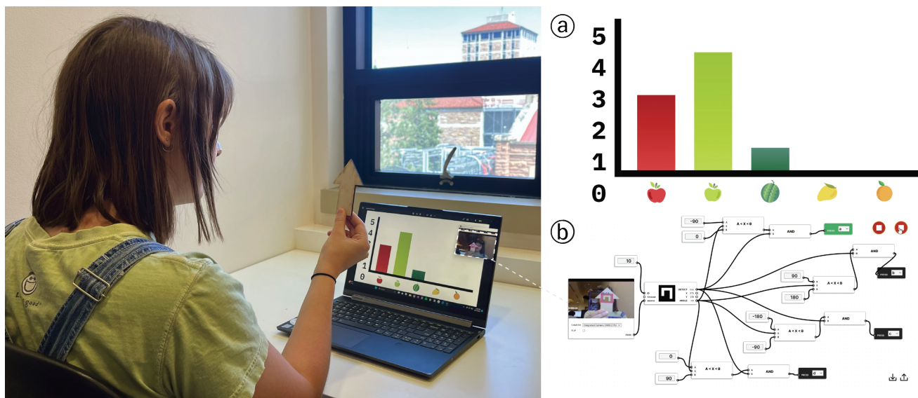
Figure 1: Embodied interactions enable a user to author their own bar graphs through a tangible input device. (a) The Figma board is where the user is able to create their visualizations. (b) Beholder library [11] tracks a fiducial marker on the authoring device and connects it to a keyboard interaction, which corresponds to an action on the Figma board.
