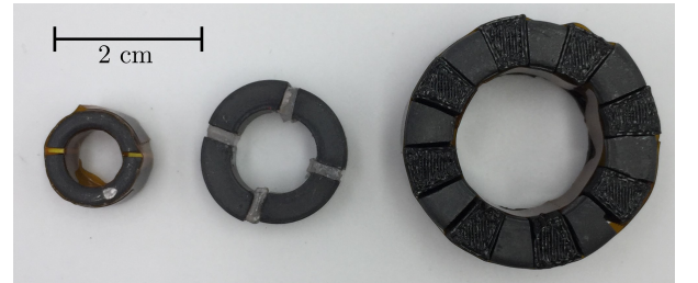
Fig. 4: Unwound toroidal cores showing implementation of quasi-distributed gaps for 10, 30, and 60 MHz.
