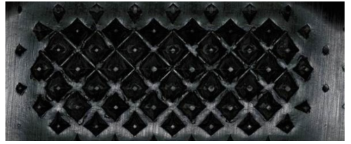
FIGURE 4: A METAL COUPON PRODUCED BY THE IMPRESSION METHOD IN [17].
