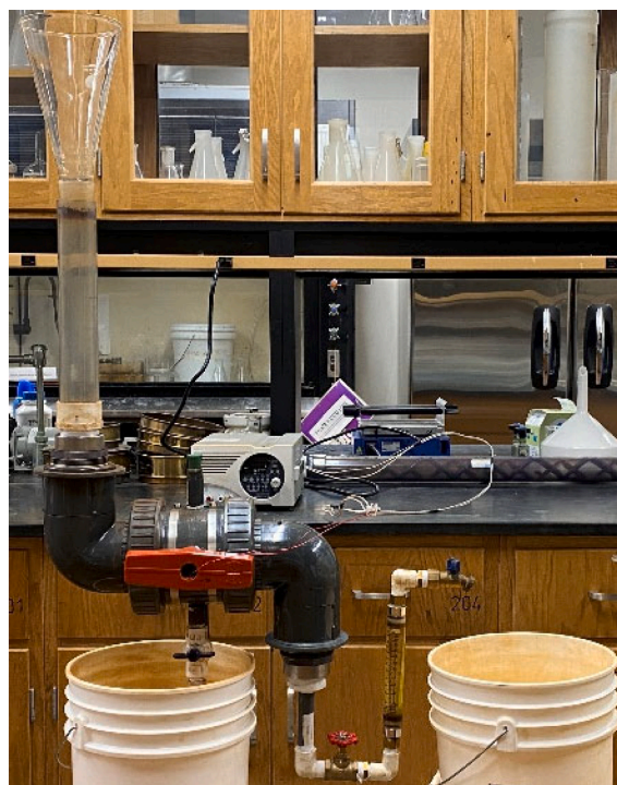
Fig. 2. Continuous flow material recovery experimental setup for flow-through operation. Schematic at left and physical setup at right.
