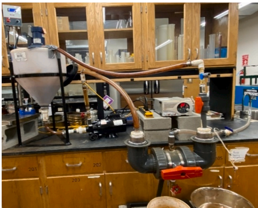
Fig. 3. Continuous flow material recovery experimental setup for continuous operation. The setup includes a mechanical mixer, feed tank, pump apparatus, electromagnet, power supply, tubing to recycle the water, and tubing to flush the electromagnet with deionized water.
