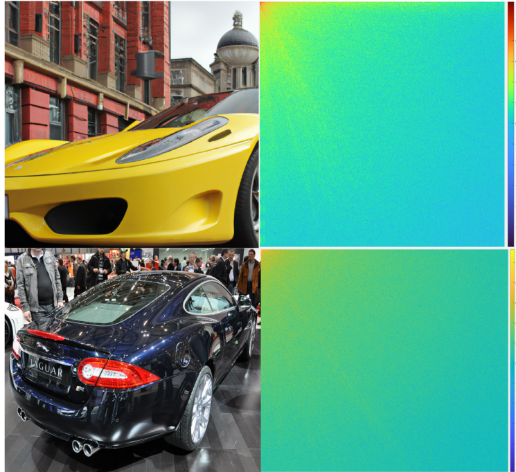
Fig 4 Row 1: Dall-E Image and its DCT. Notice the finger-like patterns at the higher frequencies. Row 2: Real Image and its DCT.
