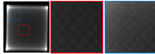
Figure 10. Lissajous scanning. Image and insets of the illumination lens' focal plane, showing the Lissajous scanning pattern.
