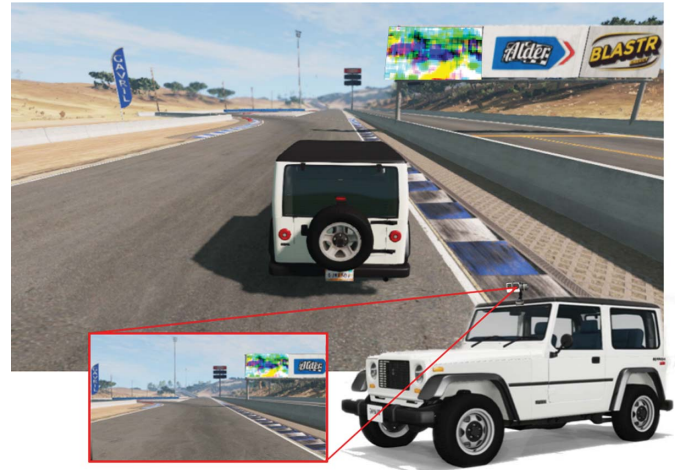
Fig. 1. Autonomous vehicle driving by a roadside billboard with perturbation generated by a patch attack.
