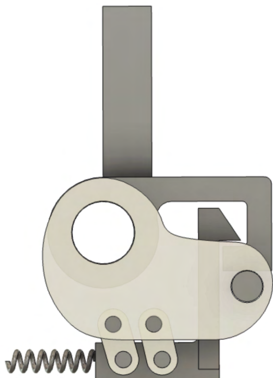
FIGURE 4: CAD MODEL OF UPDATED DESIGN OF FUNCTIONAL COMPONENTRY OF THE KNEE
