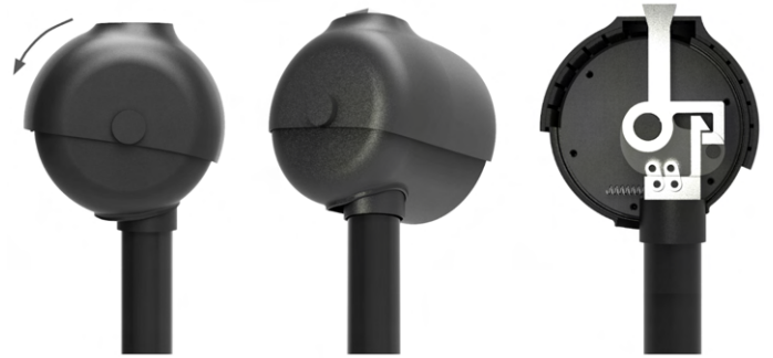
FIGURE 9: SIDE, ANGLED, AND SECTION VIEWS OF CAD MODEL OF THE ENCLOSURE
