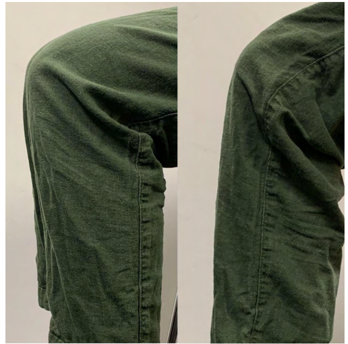
FIGURE 8: A PHYSIOLOGICAL KNEE (LEFT) UNDER PANTS, AND A PROTOTYPED PROSTHETIC KNEE ENCLOSURE (FIG. 12) UNDER THE SAME PAIR OF PANTS (RIGHT).
