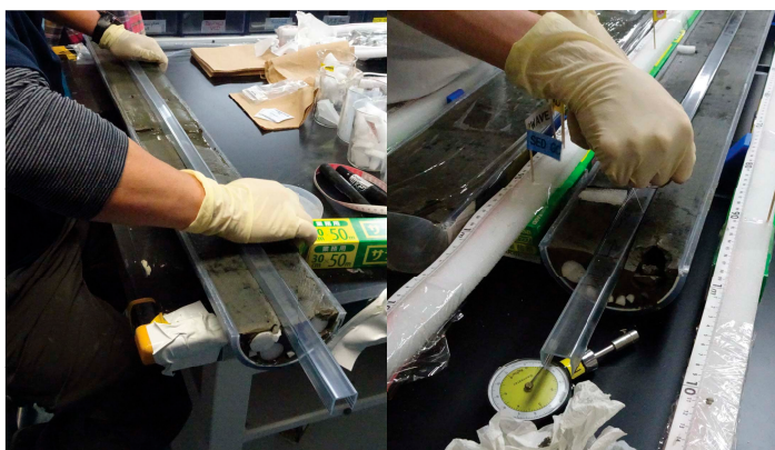
Figure F25. U-channel sampling, Expedition 386. Left: inserting U-channel into a split section. Right: cutting the U-channel from the section using fishing line.
