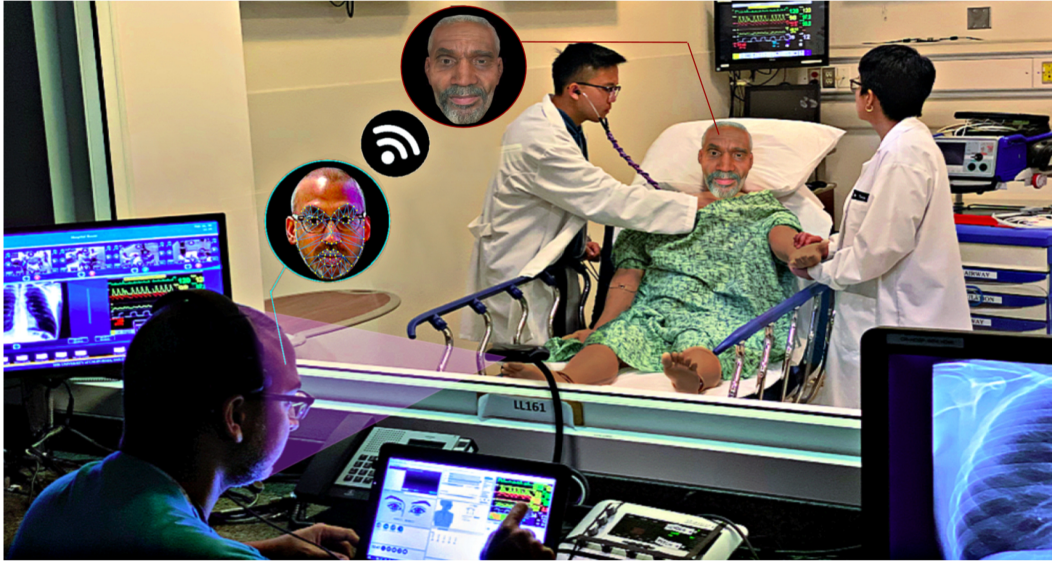
Fig. 6. Robotic patient simulators are tele-operated, life-size mannequins that can exhibit thousands of physiological signals, and can breathe, bleed, and respond to medications. However, they are largely inexpressive, leading to poor training outcomes for CLs, and possibly poor clinical outcomes for patients. Our work addresses this gap by introducing patient simulator systems with a much wider range of expressivity, including the ability to express pain, neurological impairment (e.g., stroke, Bell's Palsy), and other clinically relevant expressions, via simulators with diverse genders, races, and ages.
