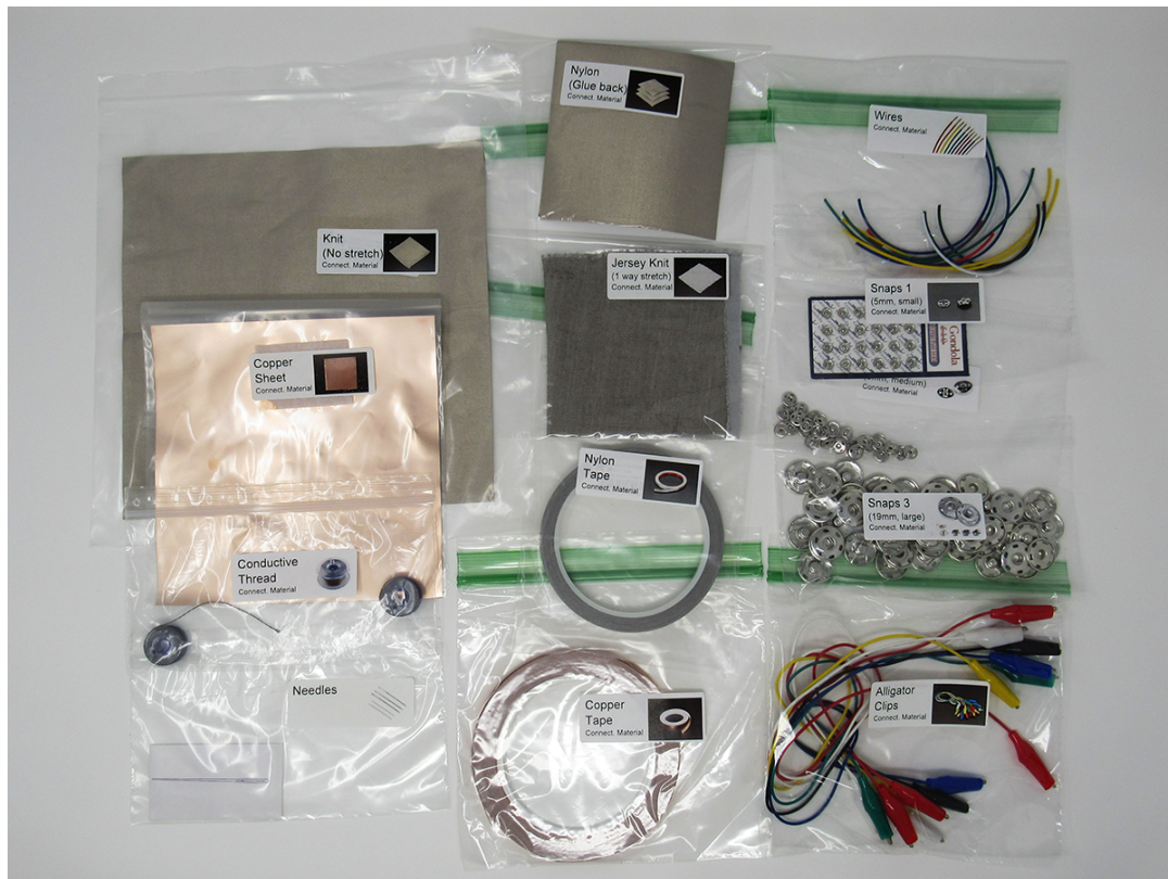
Figure 14: Bagged conductive components included in the box, demonstrating how each component was individually bagged and labeled with a colored label.
