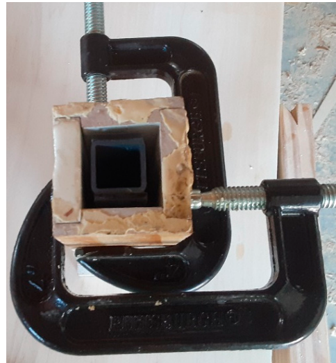
Figure 4. The final mold has been assembled, including clamping into place.
