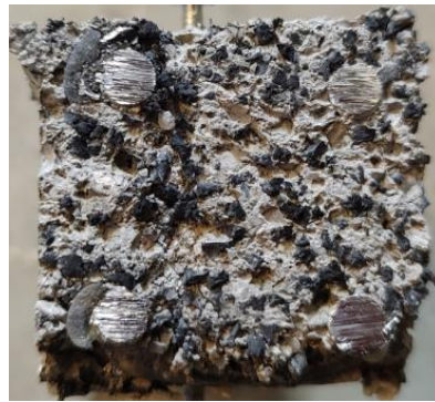
Figure 1. An example beam cross-section showing the recycled crumb rubber infill proportion. The high volumetric ratio of the crumb rubber can be seen.
