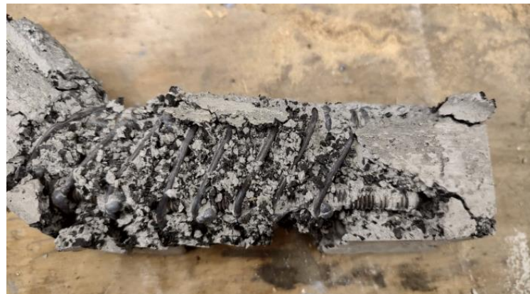
Figure 11. The failed RC-9 beam is shown.
