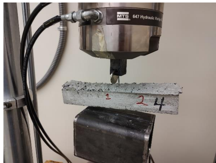
Figure 8. The nail withdrawal or pullout test setup is run in reverse to measure the force required to insert a nail into the rubber concrete and the wood. The red numbers shown indicate testing locations while the black number 4 indicates RC-4.
