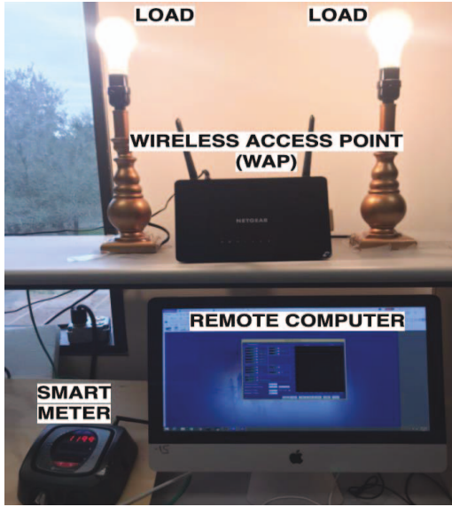
Figure 7. Experimental set up displaying the Electric Smart Meter, deployed load, wireless access point (WAP) and the monitoring remote computer.
