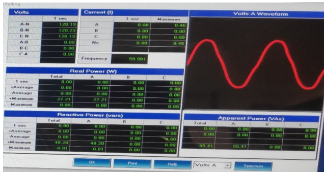
FIGURE 3. GE communicator software for data analysis and configuration used by remote monitoring computer.
