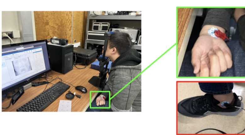
Figure 3: Experimental Setup . The left image shows the entire setup, the images on the right show placement of electrodes on subject for recording ECG. The red box illustrates electrode placement on the subject’s foot (out of view in the left picture).
