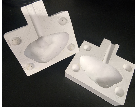
Figure 1. The 3D printed mold used to create the children phantoms. The mold was printed in two sections separated with respect to the sagittal plane allowing the gelatin phantom to be extracted.
