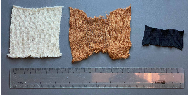
Figure 7: One instance of the half-gauge rib swatch from the Tamm Petit acrylic, Winning rayon, and Yeoman Elastomeric yarn training sets. The rayon swatch appears looser because of the lower bending stiffness of the thin rayon yarn. The elastomeric sample is smaller because the yarn stretches under the tension of knitting and contracts once released from the needles.
