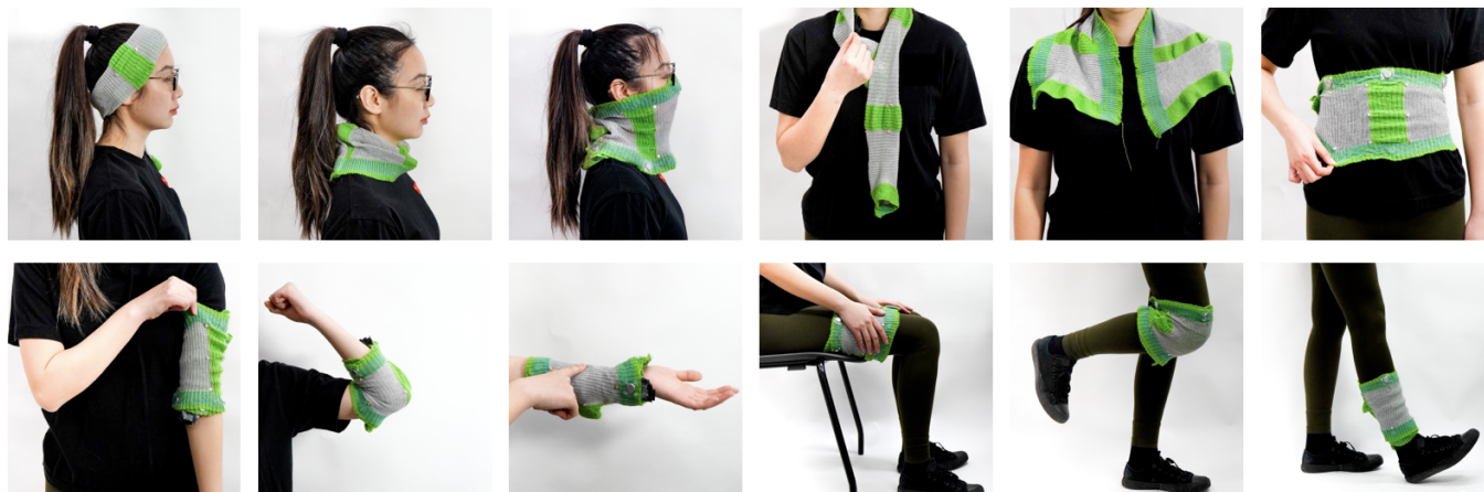
Figure 1: uKnit is a scarf-like reconfigurable wearable which can recognize its current body location placement and perform a variety of gesture recognition and sensing tasks.
