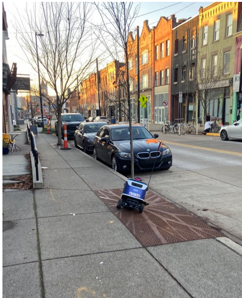
Figure 7. A PDD stuck in a grate requires human assistance to regain mobility.
