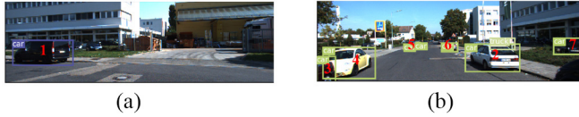
Fig. 12. Object detection results of the images collected by the cameras of the (a) ego vehicle and (b) vehicle 1.
