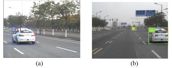
Fig. 20. Object detection results of the images collected by the cameras of the (a) ego vehicle and (b) vehicle 1 in the real-world experiment.
