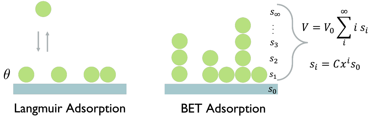
Figure 2: Langmuir model vs BET model. The BET model, unlike Langmuir, allows particles to create infinite layers on top of previously adsorbed particles. Here \theta is fraction of the surface adsorbed, V is total volume adsorbed, V_0 is the volume of a complete unimolecular layer adsorbed in unit area, s_i is the surface area of the i^{\text{th}} layer, s_0 is the surface area of the zeroth layer, and x and C are constants that relates heats of adsorption of the molecule in layers.
