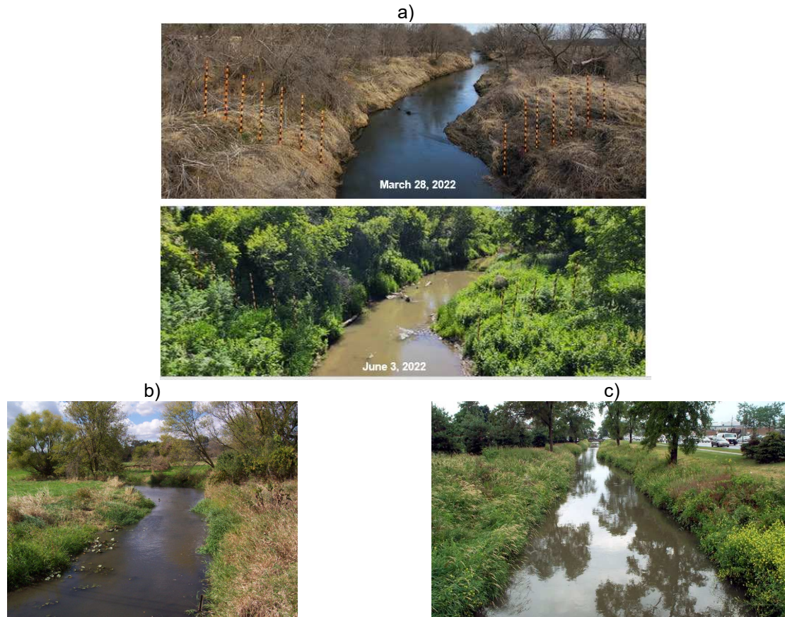
Figure 6. Vegetation growth monitored by webcam #2 at Clear Creek site (USGS stage sensor location), bed slope 0.0004. a) vegetation status before the start of the growing season (March 28, 2022) and during the growing season (June 3, 2022); b) n = 0.047 for Mill Creek (IL), bed slope 0.00047 (September 2004); and, c) n = 0.047 for Rayse Creek (IL), bed slope 0.00044 (September, 1999)
