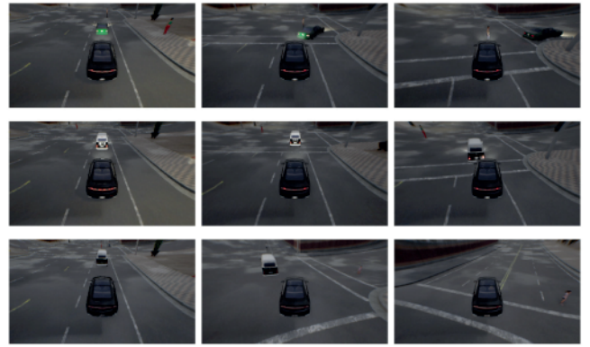
Fig. 5. RQ1. Example traffic violations found by AutoFuzz . For each row, the time goes by from left to right. (1st row) pid-1 controller collides with a pedestrian crossing the road. (2nd row) pid-2 controller collides with the stopped leading car. (3rd row) lbc controller makes a wide turn into the opposing lane (considered "off-road").
