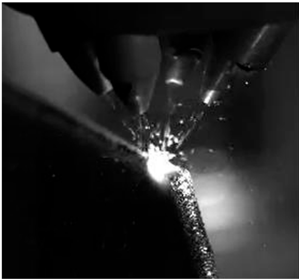
FIGURE 4 High speed camera image during a metal directed energy deposition process.
