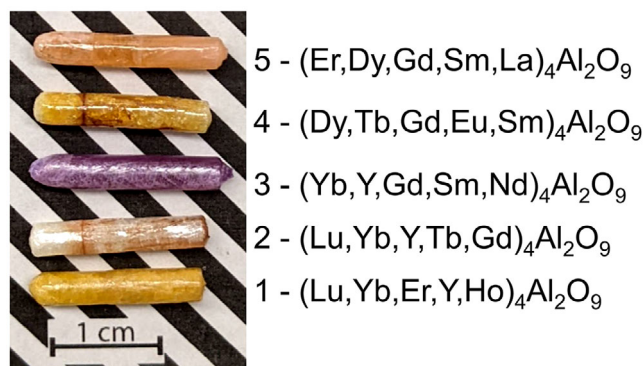
FIGURE 1 Photo of the high-entropy RE 4 Al 2 O 9 crystals. Composition ID is indicated in the figure and refers to the composition in Table 2. Crystals are 3 mm in diameter and were grown with good shape control. All crystals were polycrystalline at room temperature.
