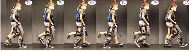
Fig. 7. Gait tiles of human-prosthesis multi-contact walking. Experimental results from Gehlhar and Ames (2023) showing the resultant multi-contact behavior obtained by developing trajectories with a multi-domain hybrid system. Labels correlate with domains in Fig. 6.
