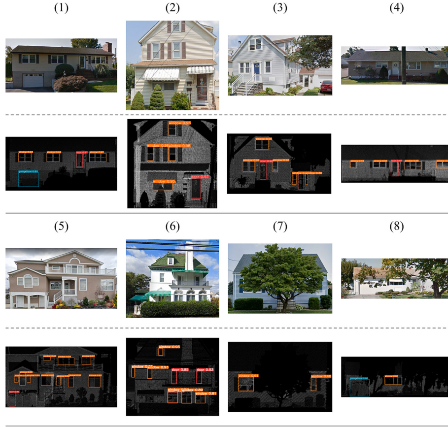
Fig. 4. Visual inspection of the object detection results. The first and third rows display Google Street View images, while the second and fourth rows depict intensity-based front views with detected bounding boxes.
