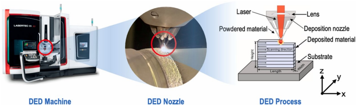
Fig. 1. DED process diagram; part width in y direction is equivalent to one laser diameter, making the part “thin-walled”. adapted from DMG Mori, Optomec, and (Zhang et al., 2020)
