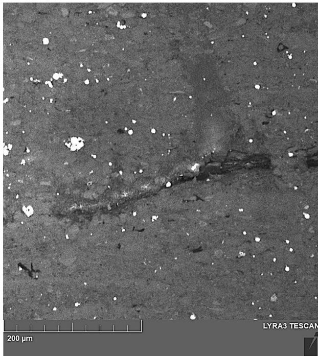
Fig. 22 SEM-BSE image displaying the merging of microcracks and the development of a larger crack, evident across the depth of the 28-day reacted sample
