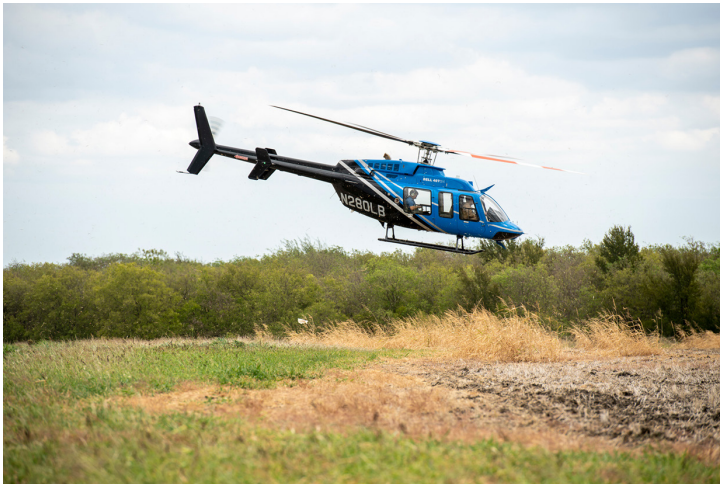
Test flights in October 2022 were conducted to evaluate communications technologies that could be used to guide future vertical-takeoff aircraft in urban settings. Although the future aircraft will likely be electric, for the tests organizers flew a Bell 407GX helicopter.
