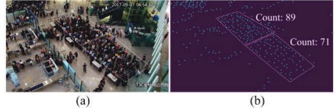
Fig. 1. (a) Representative images of CS data set [11]. (b) Representative images of ground-truth of the density map. By integrating the density map, we can easily get the number of people in any region.
