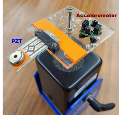
Fig. 3. Shaker platform with the accelerometer and PZT cantilever mounted.
