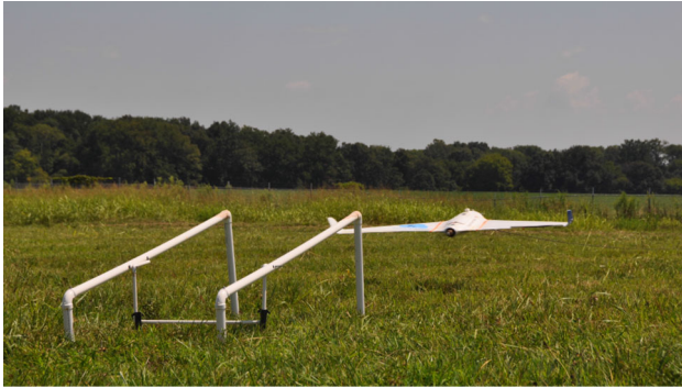
Fig. 4 UAV during catapult-assisted launch
