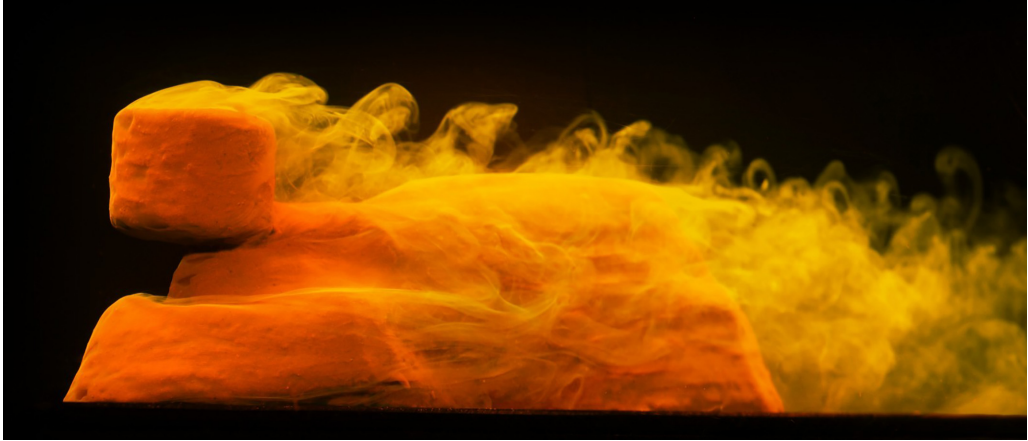
FIG. 1. A laboratory Sphinx in the current of a water tunnel. The object is coated with clay and fluorescein dye, and the photograph captures the “streak volume” or 3D region of flow that has at some time entered the boundary layer and eroded the surface.
