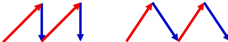
Fig. 2. Schematic representation of heating (red arrows) and cooling (blue arrows) patterns used for viscosity cycles. Sawtooth (left) and triangle (right) patterns are shown for two cycles.
