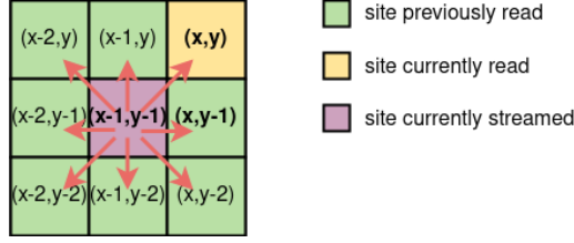
Figure 2: Illustration of the staggered lattice update. When the update loop arrives at site (x, y) , the sites with lower indices (green and purple) have already been read. Once the site (x, y) (yellow) has been read, site (x - 1, y - 1) (purple) can be streamed to its neighbors. The illustration shows the situation in 2D; the generalization to 3D is straightforward.
